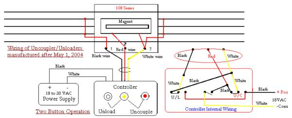
NOTE: YELLOW BUTTON MUST ALSO BE PUSHED ALONG WITH EITHER Uncouple or Unload Button to Operate
